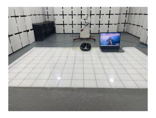
Set-up for Radiated Spurious Emission, Above 1GHz
