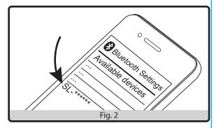
Check the list of available devices on the Bluetooth® device to see if "SL-\*\*\*\*\*" (where \* stands for a unique number) is detected. The list may need to be refreshed, or manually scanned for new connections. Select the "SL-\*\*\*\*\*" name to pair device with the fixture. Once connection is established, the fixture speakers will emit a single chime.
