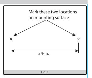
Drill pilot holes in each of the two marked locations.
