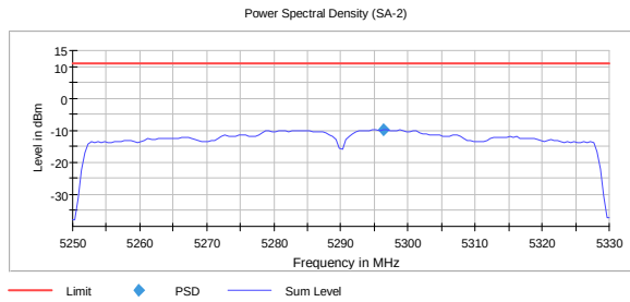
PSD, 5290 MHz, 802.11ac, HT80, MCS0 -9.7 dBm
