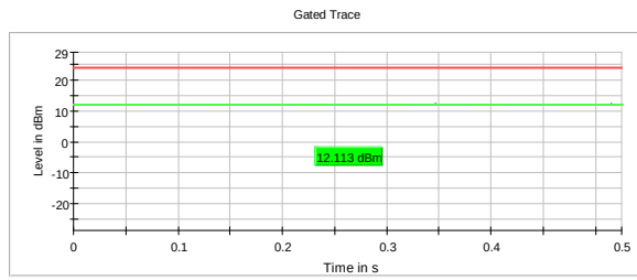
RMS Conducted Power, 5720 MHz, 802.11ax, HT20, MCS0, MIMO
