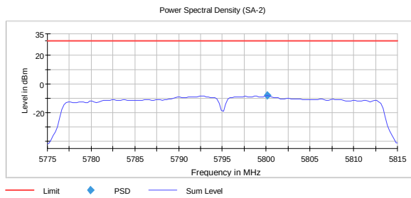
PSD, 5795 MHz, 802.11ac, HT40, MCS0, MIMO -8.2 dBm
