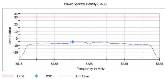
PSD, 5825 MHz, 802.11n, HT20, MCS8, MIMO -5.4 dBm
