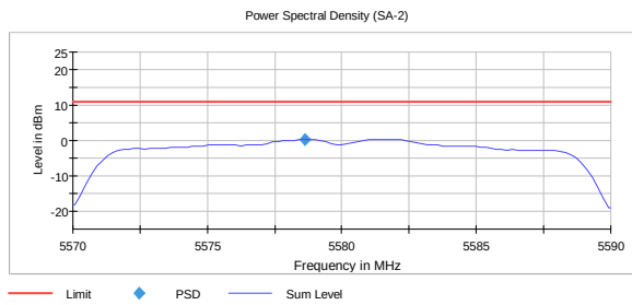
PSD, 5580 MHz, 802.11n, HT20, MCS8, MIMO 0.3 dBm
