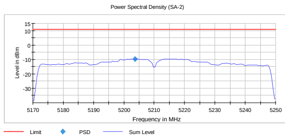
PSD, 5210 MHz, 802.11ac, HT80, MCS0 -9.7 dBm
