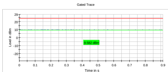
RMS Conducted Power, 5260 MHz, 802.11ax, HT20, MCS0, MIMO
