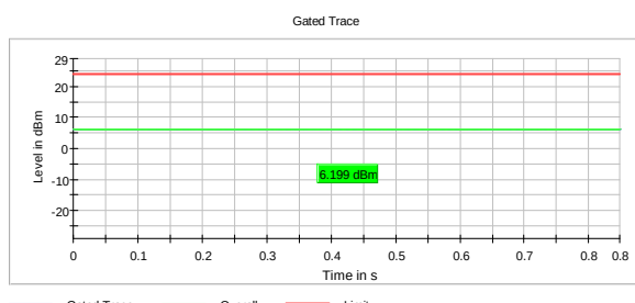
RMS Conducted Power, 5310 MHz, 802.11ax, HT40, MCS0, MIMO
