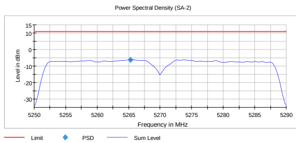
PSD, 5270 MHz, 802.11ac, HT40, MCS8 -6.1 dBm
