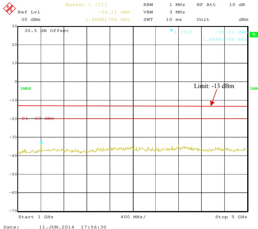
**Digital Modulation:****30MHz - 1 GHz, 450.0125 MHz for FCC Part 74/90**
