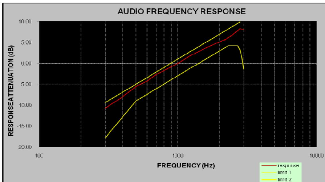
**Audio Frequency Low Pass Filter Response****Analog Modulation:**
