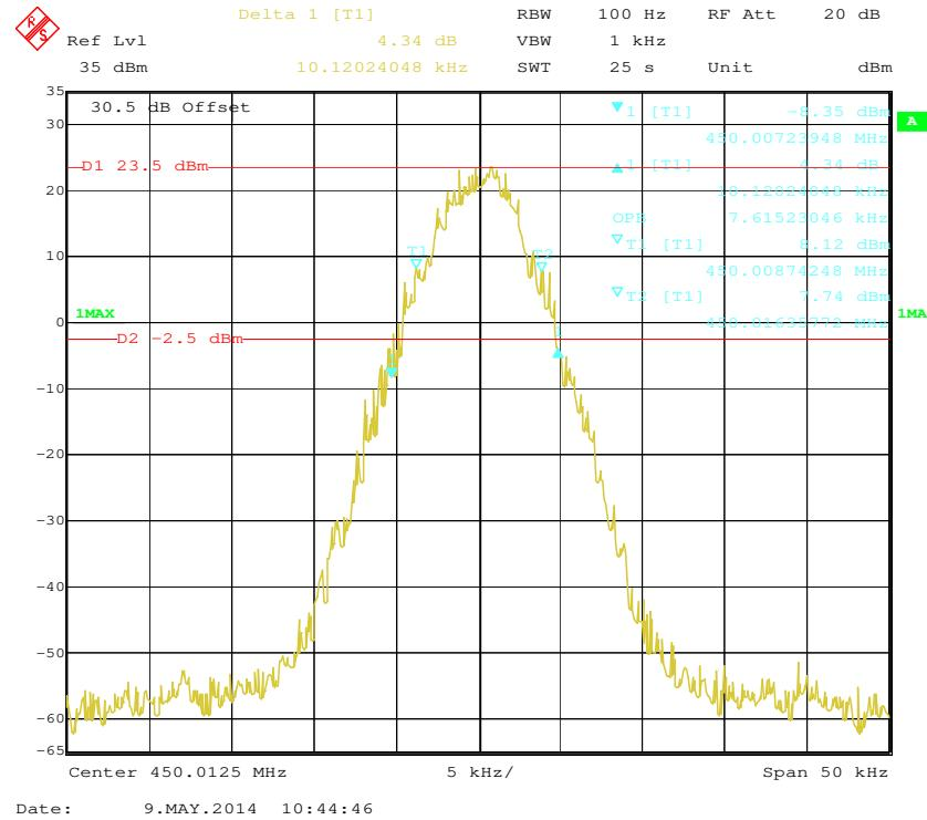
**Digital Modulation: Emission Mask with High Power**
