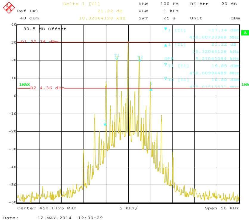
**Analog Modulation: Emission Mask with High Power**
