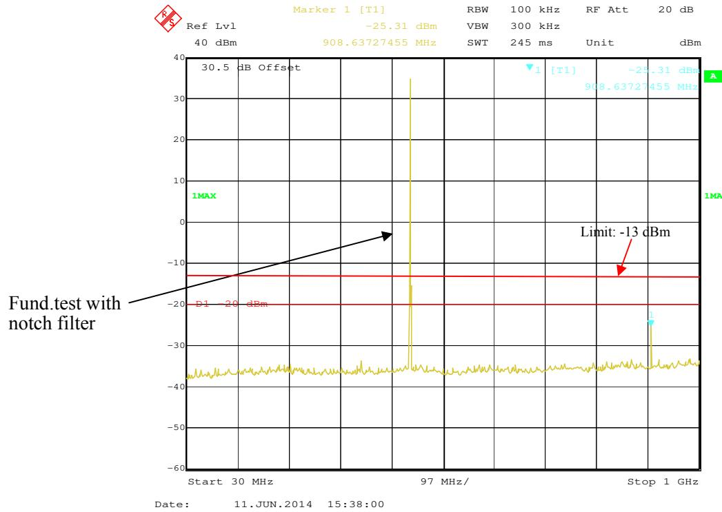
**1 GHz – 5 GHz, Spacing Channel 12.5 kHz, 454.0125 MHz for FCC Part 22**
