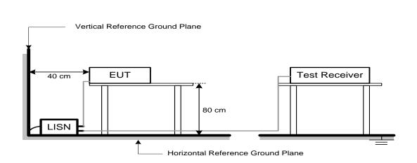
The LISN edge is arranged parallel to the edge of the test table The vertical conducting plane or wall of an RF-shielded (screened) room shall be located 40 cm to the rear of the EUT
