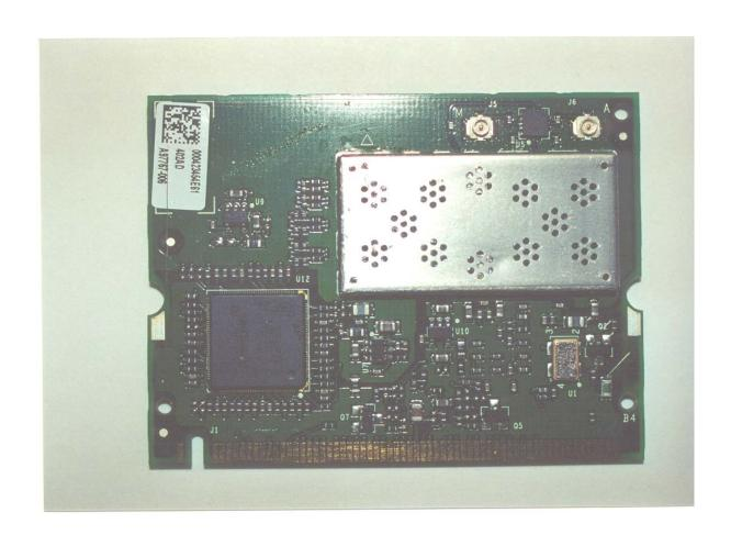
Top View of the WLAN Transmitter "Insulation removed"
