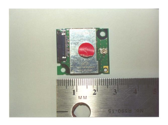
Top View of Bluetooth Transmitter "With Shield"
