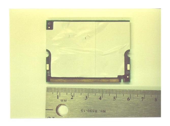
Bottom View of the WLAN Transmitter "Insulation Added"
