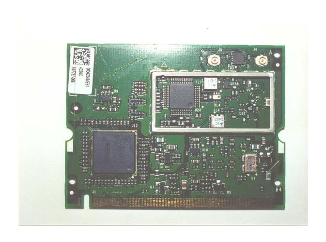
Top View of the WLAN Transmitter "Shielding removed"
