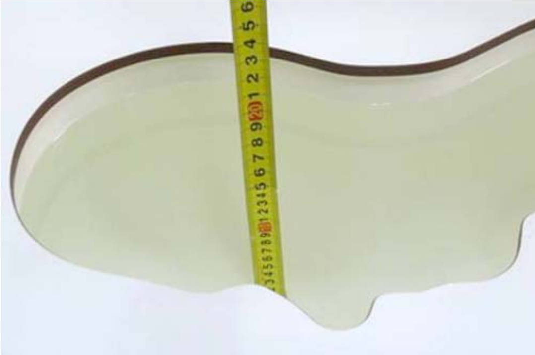
Picture 3: liquid depth in the head Phantom
