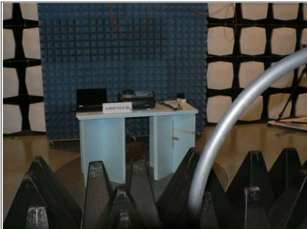
Photograph 4: Radiated measurements test set-up for magnetic fields
