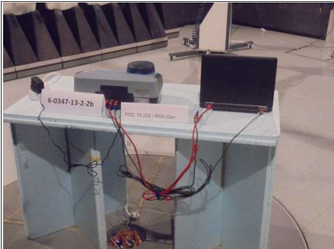
Photograph 3: Radiated measurements test set-up
