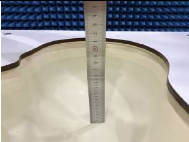
Fig. 9.7 Photo of Liquid Height for Head SAR (5200MHz~5800MHz) (depth>15cm)
