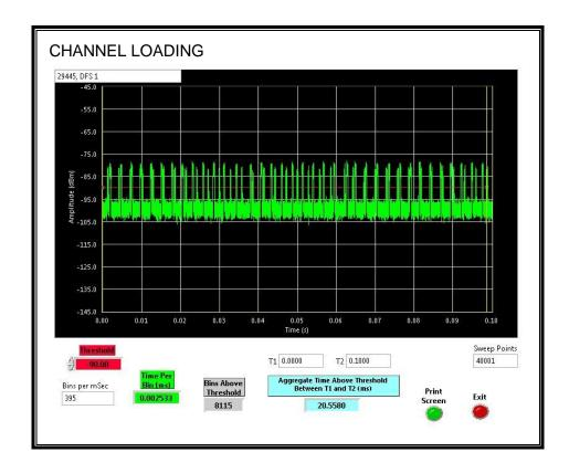
The level of traffic loading on the channel by the EUT is 20.55%
