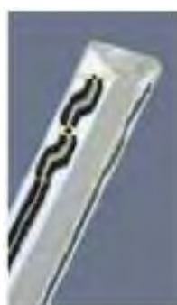
Figure 4.3 Probe Thick-Film Technique
