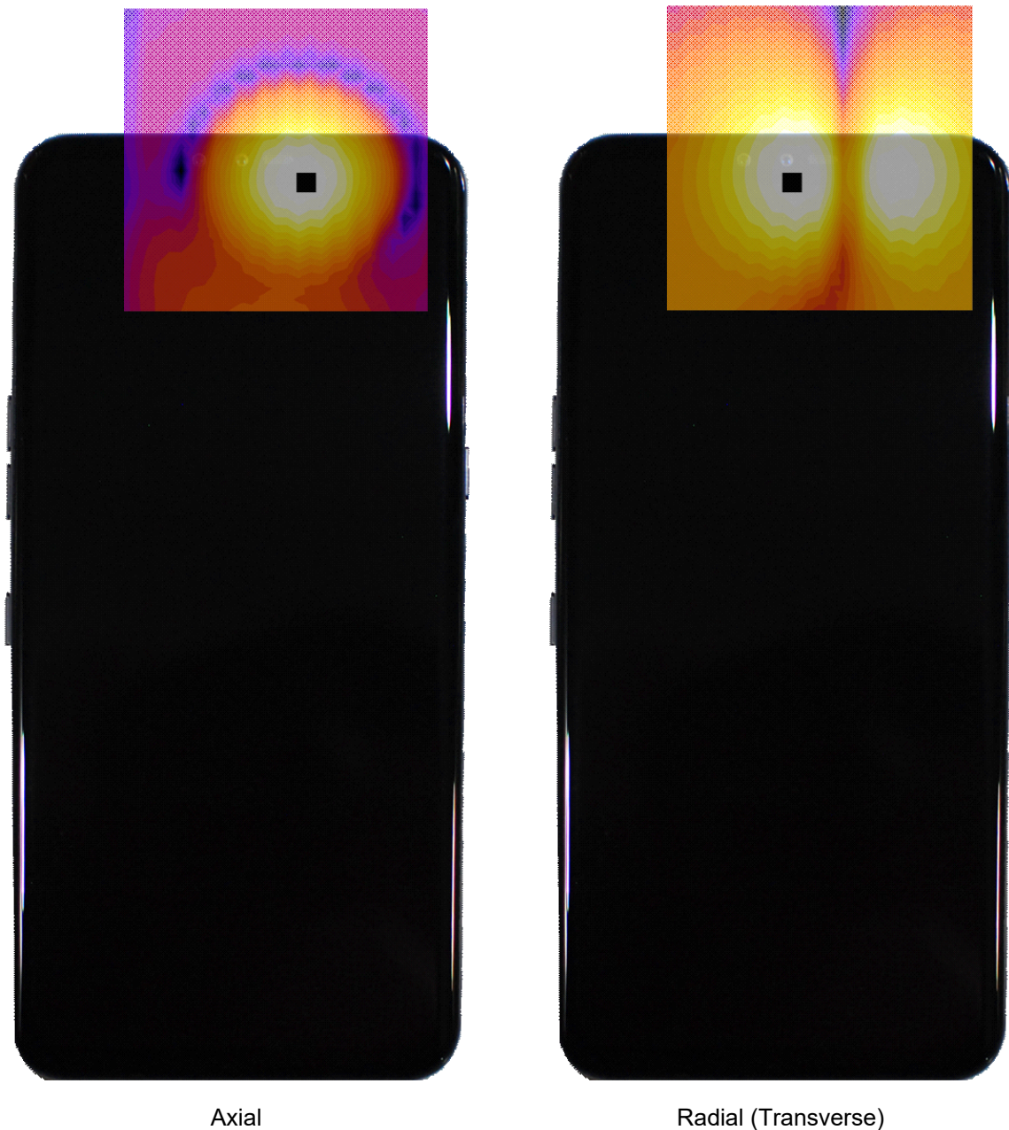
Figure 16-3 T-Coil Scan Overlay Magnetic Field Distributions
