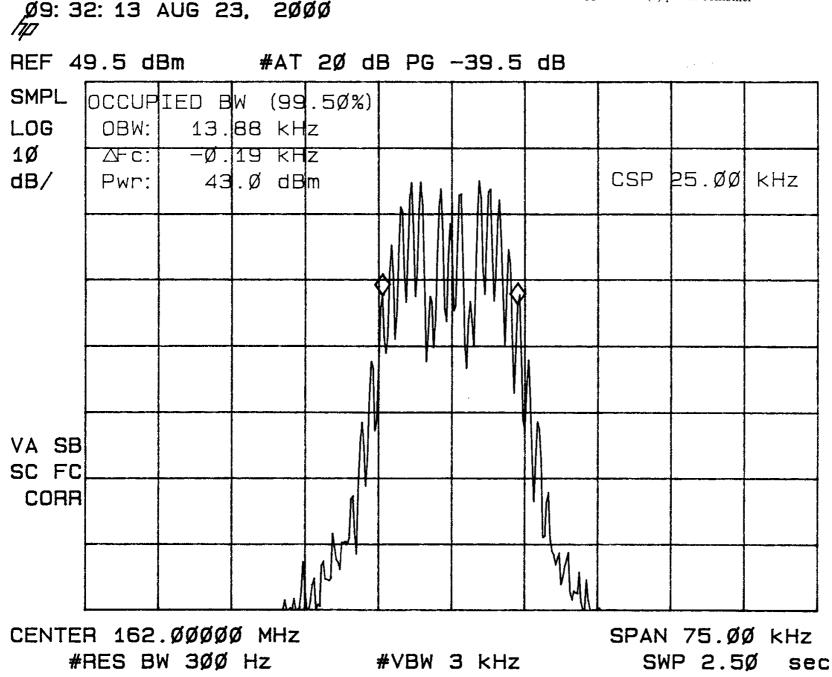
CLIENT: CUBIC COMMUNICATIONS SPECIFICATION: Part 2, Paragraph 2.1051; Part 80, Paragraph 80.211 NOTE(S): 1. Low channel (conducted spurious) 2. EUT consists of: (8) MTC-100
