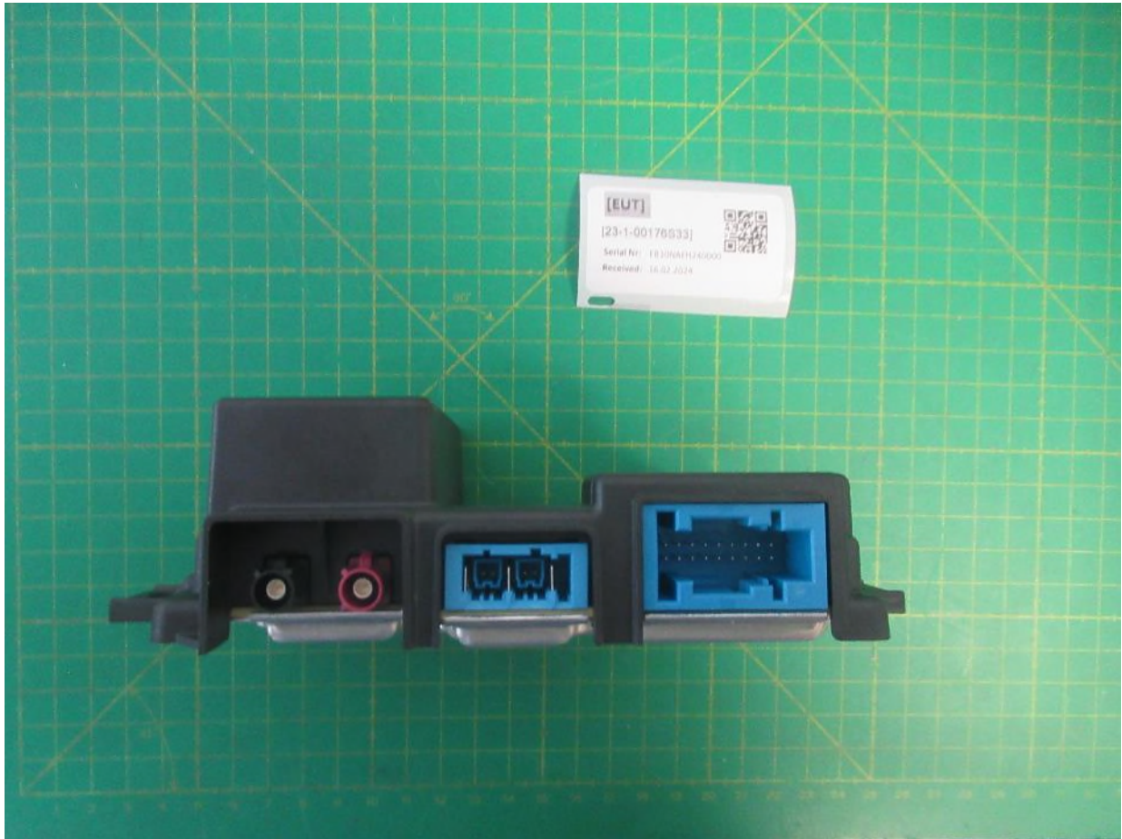
Fig. Ext.: 6 : Ext. - Special Emergency call control unit
