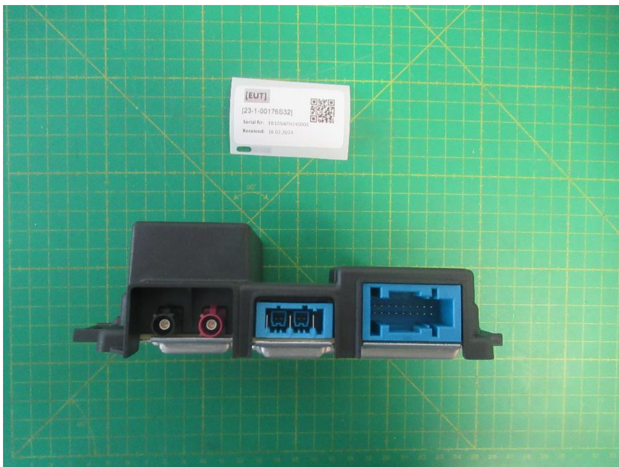
Fig. Ext.: 4 : Ext. - Special Emergency call control unit
