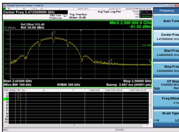
,Plot 2,Band Edge-802.11b,2462MHz ,Ant0
