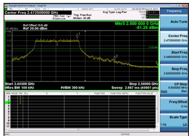
,Plot 2,Band Edge-802.11g,2462MHz ,Ant1
