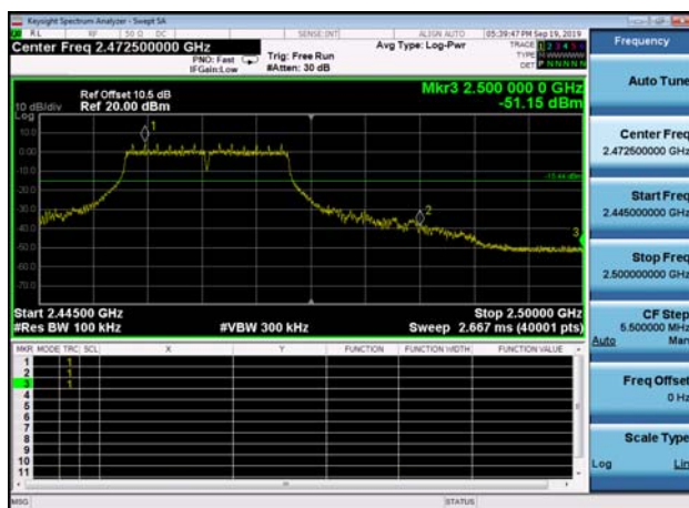
,Plot 2,Band Edge-802.11g,2462MHz ,Ant0
