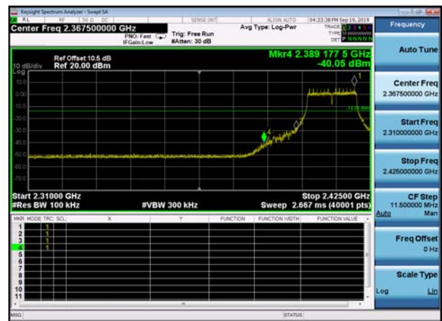
,Plot 2,Band Edge-802.11g,2437MHz ,Ant1
