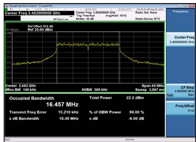
6dB Bandwidth-802.11n(HT20),2462MHz ,Ant1
