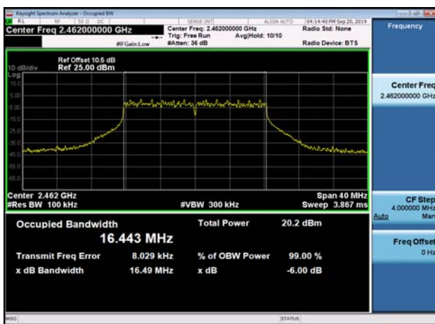
6dB Bandwidth-802.11n(HT20),2462MHz ,Ant0
