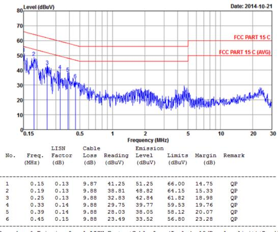
Remarks: 1.Emission Level=LISN Factor+Cable Loss(Include 10dB pulse limit)+Reading.
