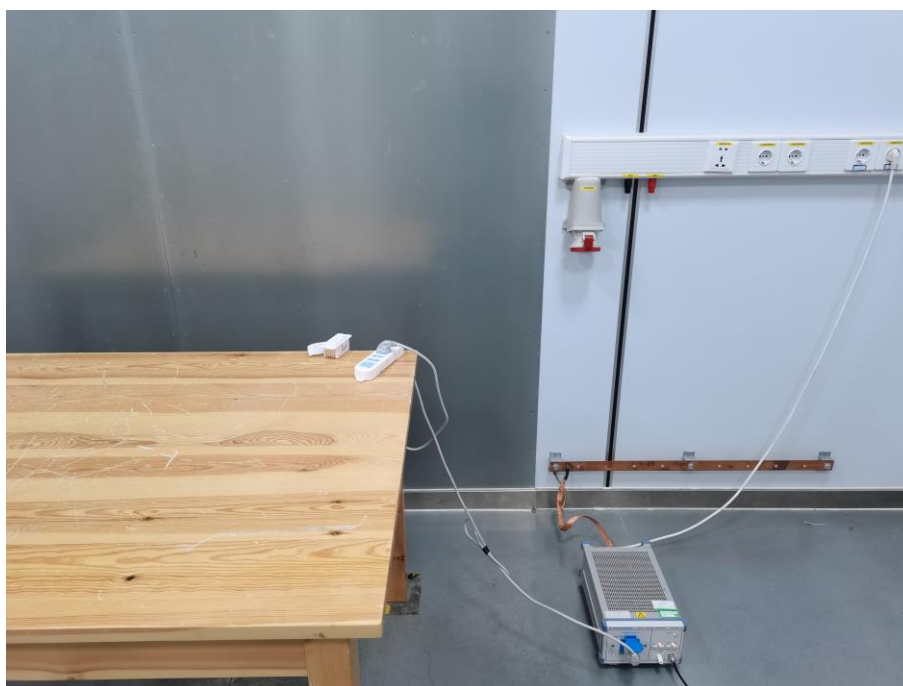
Fig. 4 Power line conducted emission setup photo
