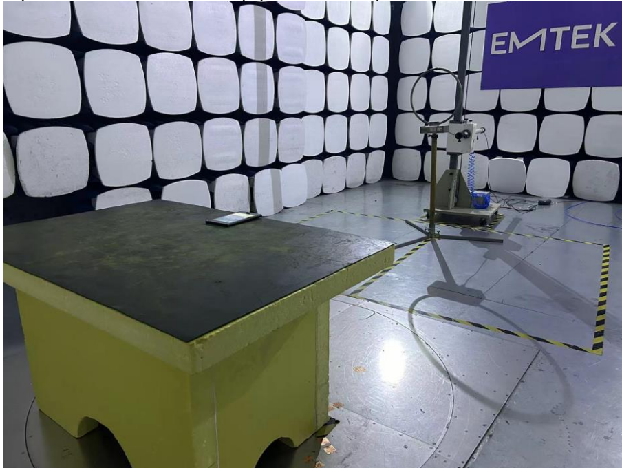
Spurious Emission Test Setup (Below 1GHz)
