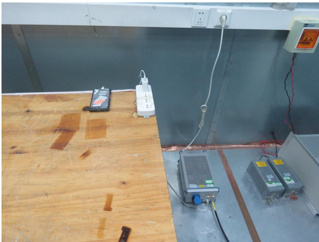
Picture 2 Conducted Emission Test Setup
