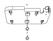
Position the access point over the mounting back plate and align the slider pegs into the slider peg holes. Carefully slide the access point downwards until the access point stops into position.
