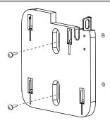
Position the access point over the mounting back plate and align the slider pegs into the slider peg holes.
