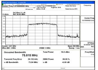
Mode:802.11ac VHT80 Frequency:5530MHz
