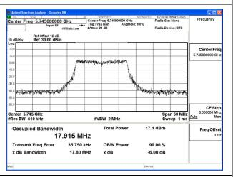
Mode:802.11ac VHT20 Frequency:5825MHz
