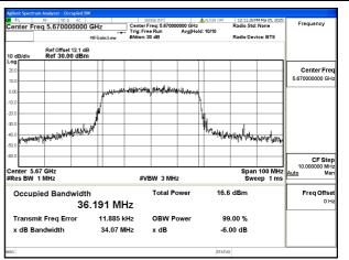
Mode:802.11ac VHT40 Frequency:5590MHz
