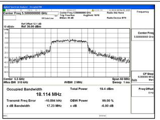
Mode:802.11ac VHT20 Frequency:5700MHz
