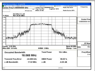
Mode:802.11ac VHT20 Frequency:5500MHz
