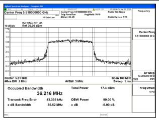
Mode:802.11ac VHT40 Frequency:5670MHz
