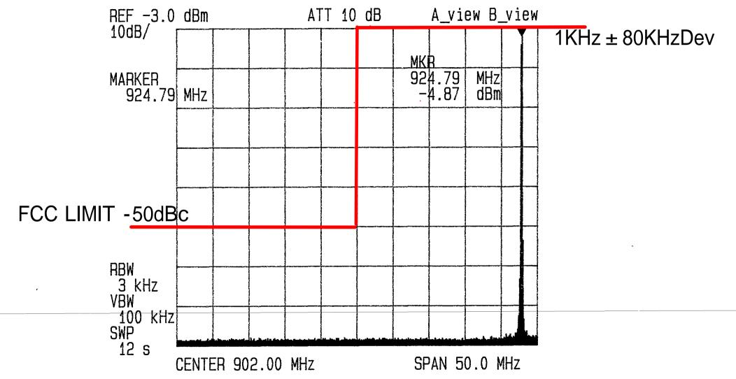
EXI3246 PORT TX Band edge emissions: CH20 MAX Dev Handset CH20
