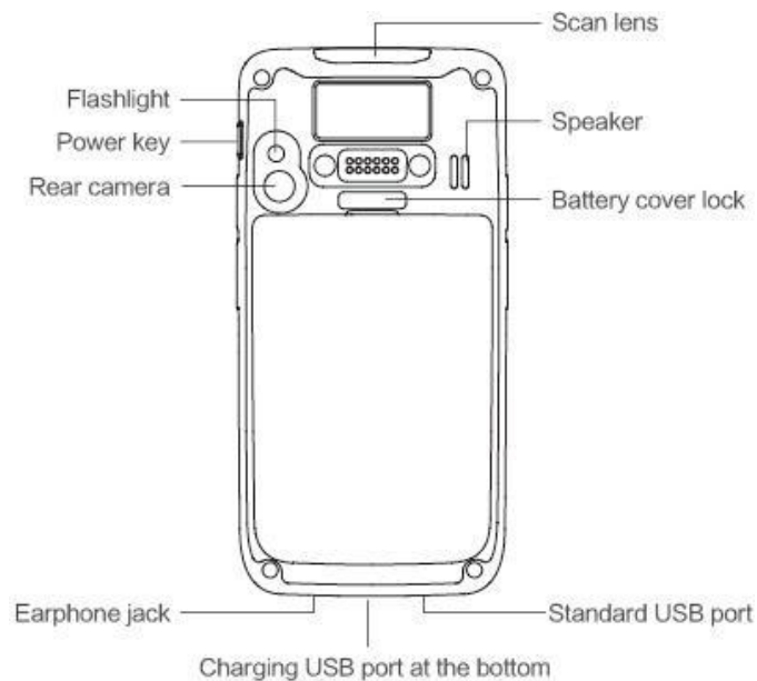
Figure 1-2 Rear view of NAUTIZ X2-V
