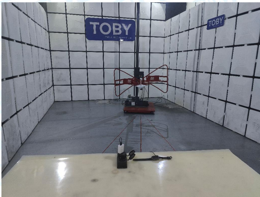
Photo of Setup for Radiated Emission (30MHz~1GHz)
