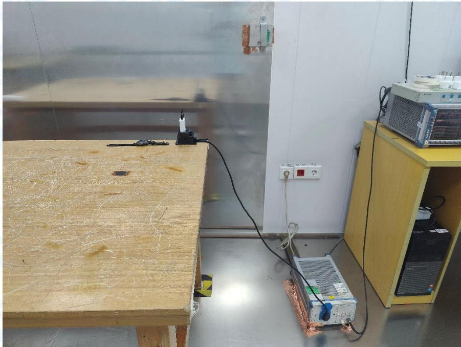
Photo of Setup for Radiated Emission (30MHz~1GHz)
