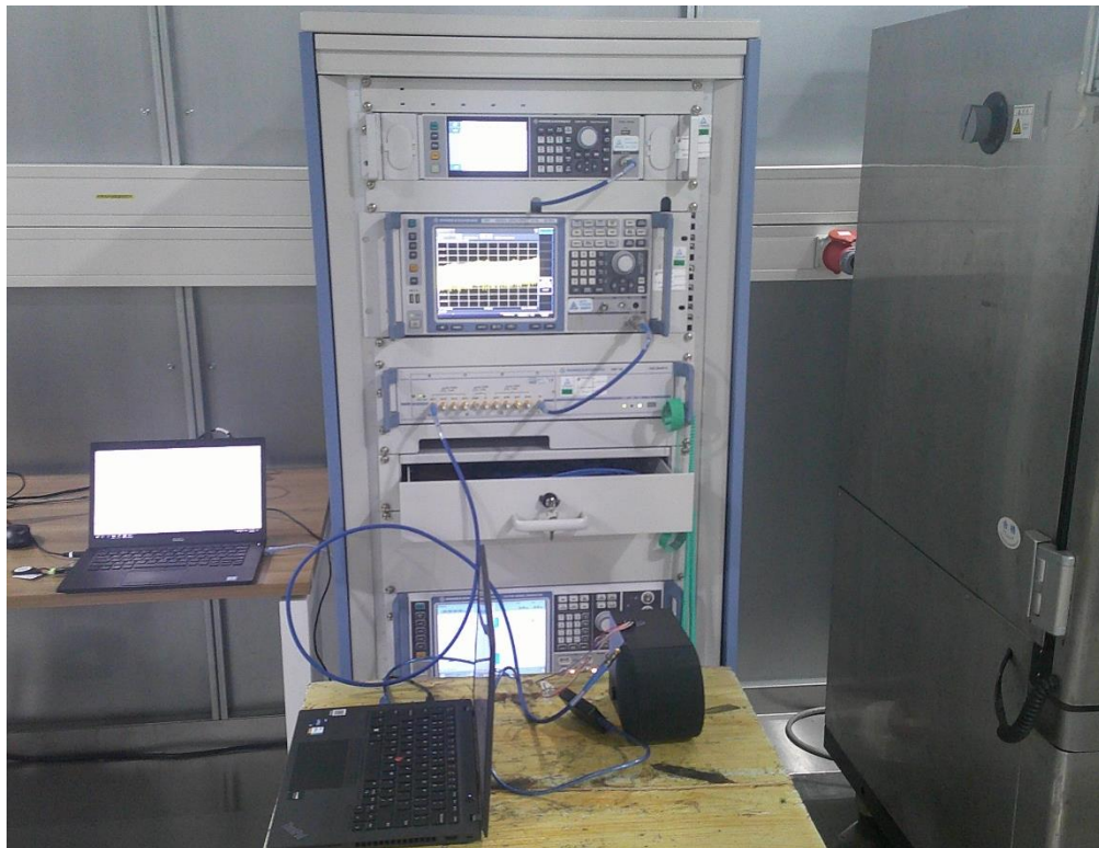
Photograph 1: Set-up photo for RF Conducted Test
