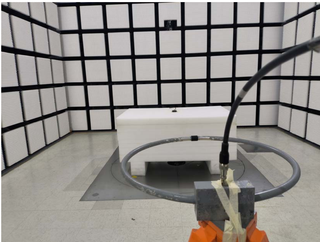
Radiated Emission 9k-30MHz View Ground-parallel
