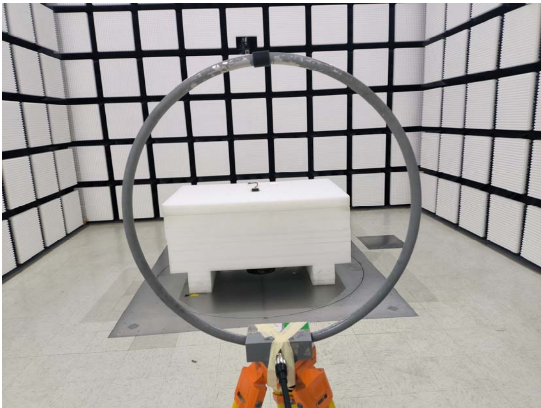
Radiated Emission 9k-30MHz View Parallel
