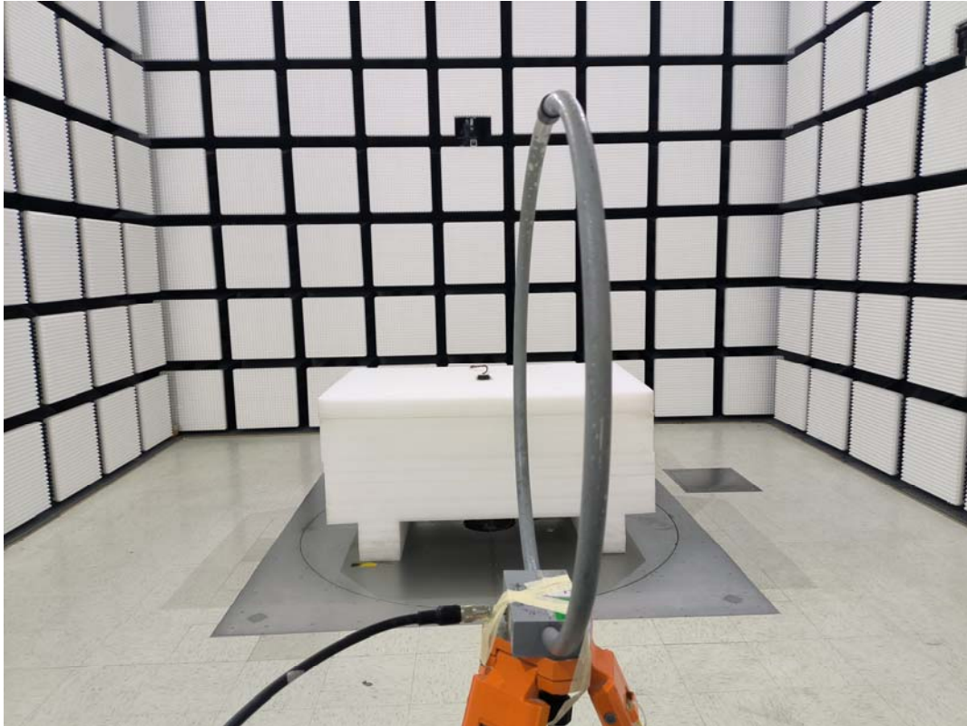
Radiated Emission 9k-30MHz View Ground-parallel
