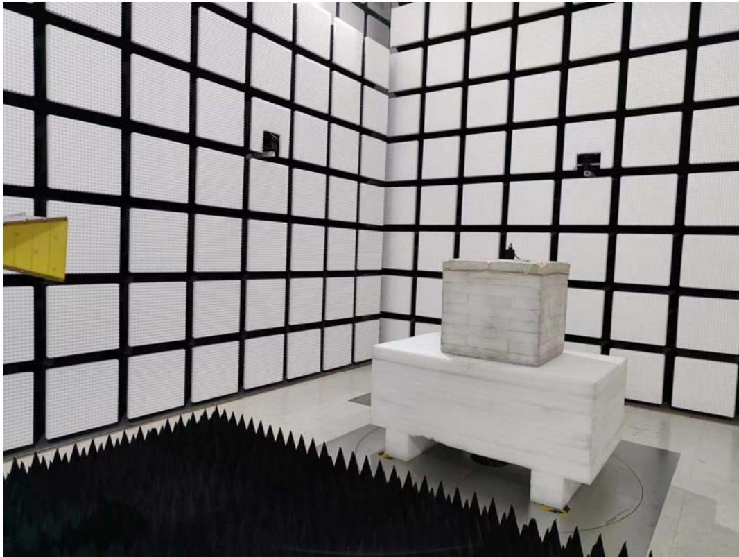
Radiated Emission Above 1GHz View 18G-26.5G
