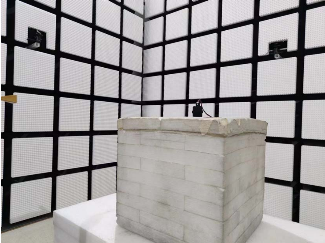
Radiated Emission Above 1GHz View 90G-140G
