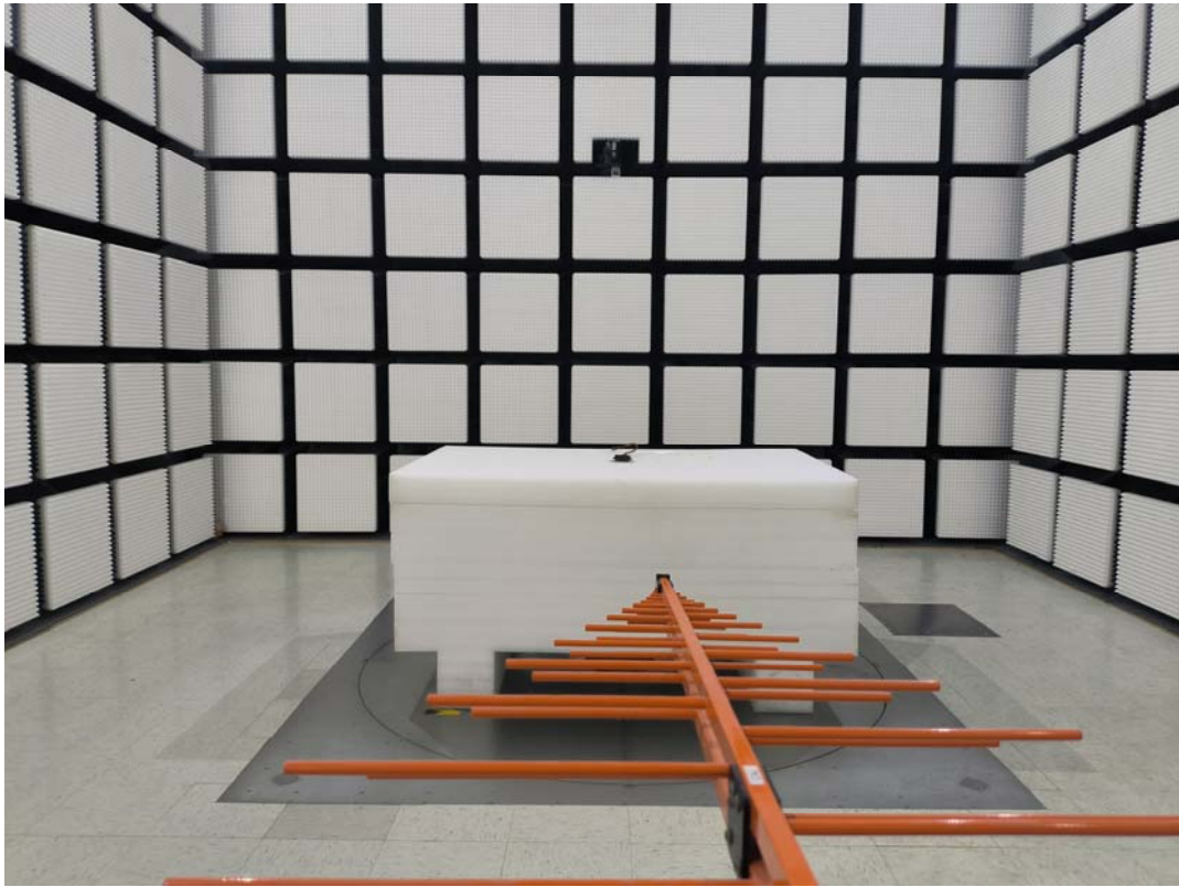
Radiated Emission 9k-30MHz View Parallel
