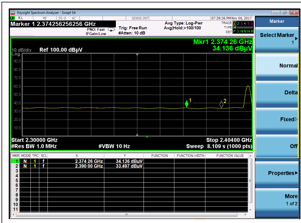
(Plot E2: Channel = 0 AVERAGE @ 8-DPSK Mode)
