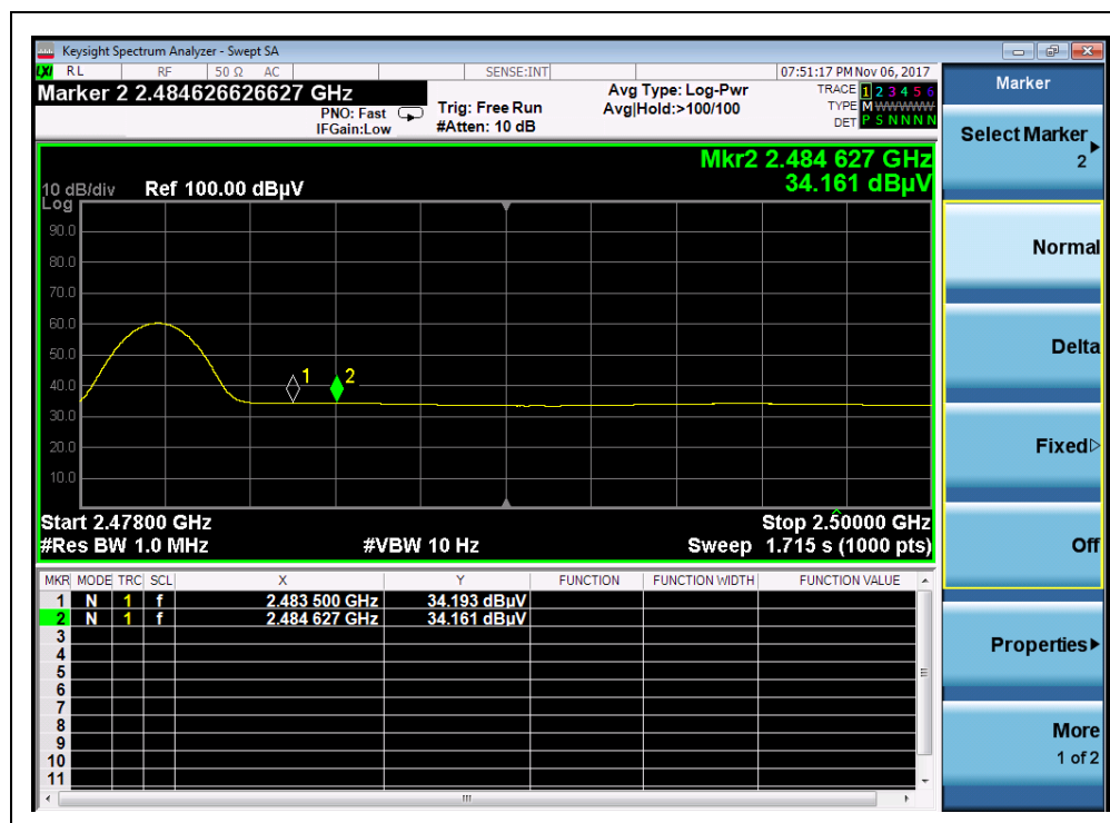
(Plot F2:Channel = 78 AVERAGE @ 8-DPSK Mode)
