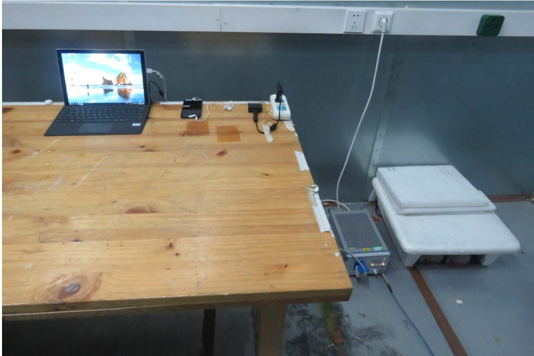
Picture 2 Conducted Emission Test Setup
