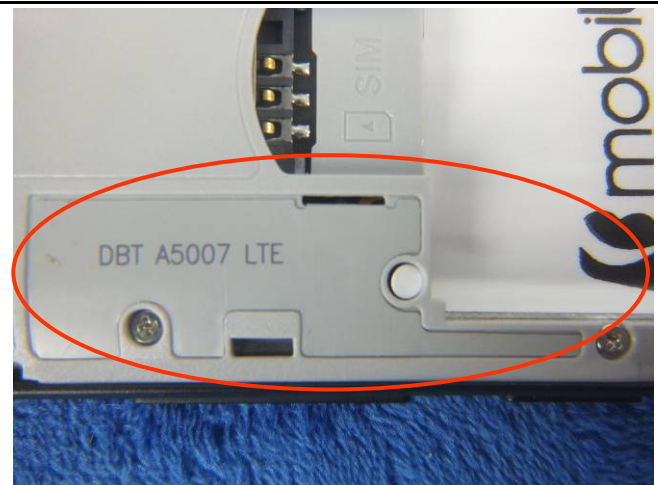
LTE- Antenna View
