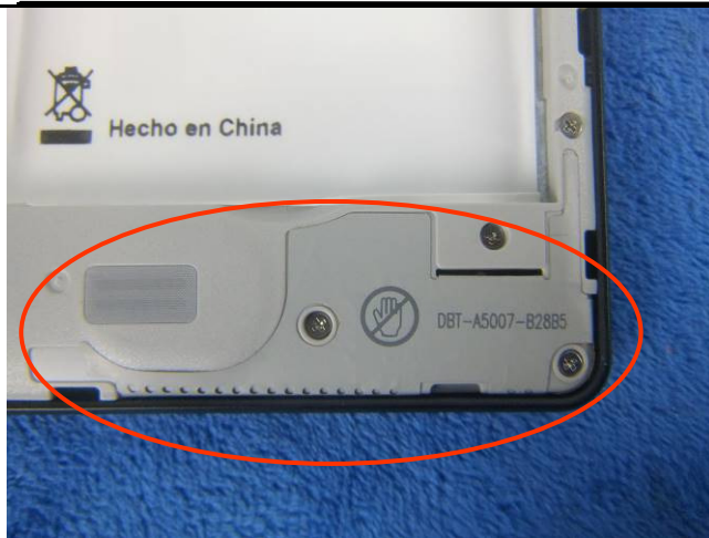
GSM/PCS/UMTS-FDD Antenna View
