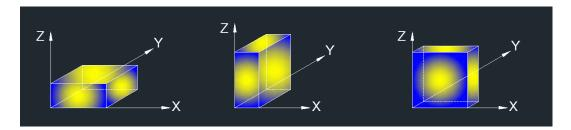
Note: For all radiated test, EUT had been tested in X axis position according to the user manual that the product should be installed in X axis position.
