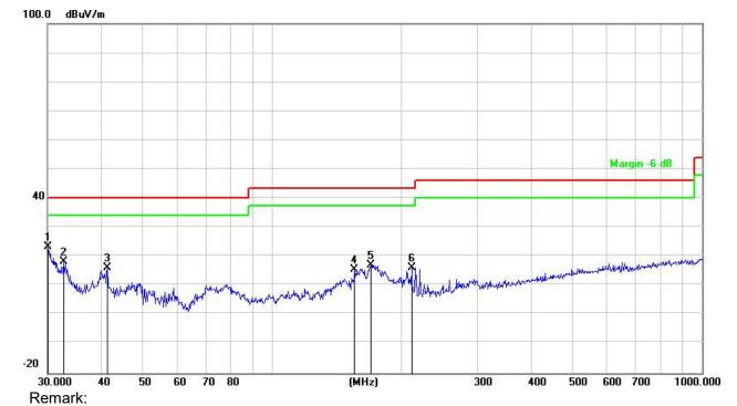
Factor = Antenna Factor + Cable Loss - Amplifier.
