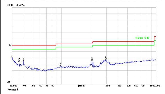
Factor = Antenna Factor + Cable Loss - Amplifier.
