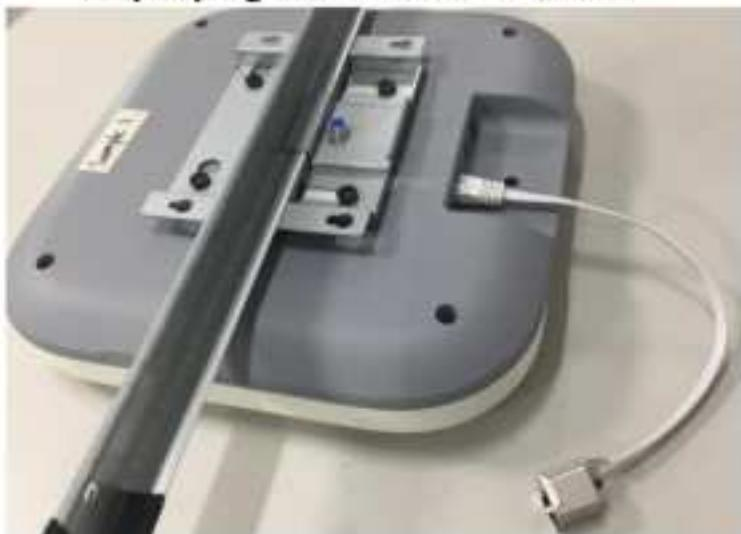
**Step2. put cable into cable slot of ceiling plate.**
