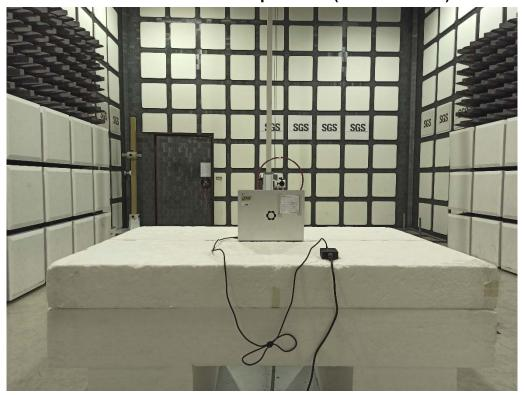
Radiated Emission Set up Photos (Below 1GHz)
