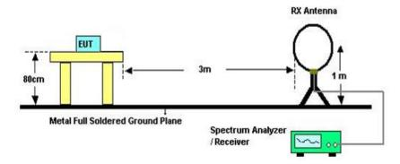
The setting of the spectrum analyzer
