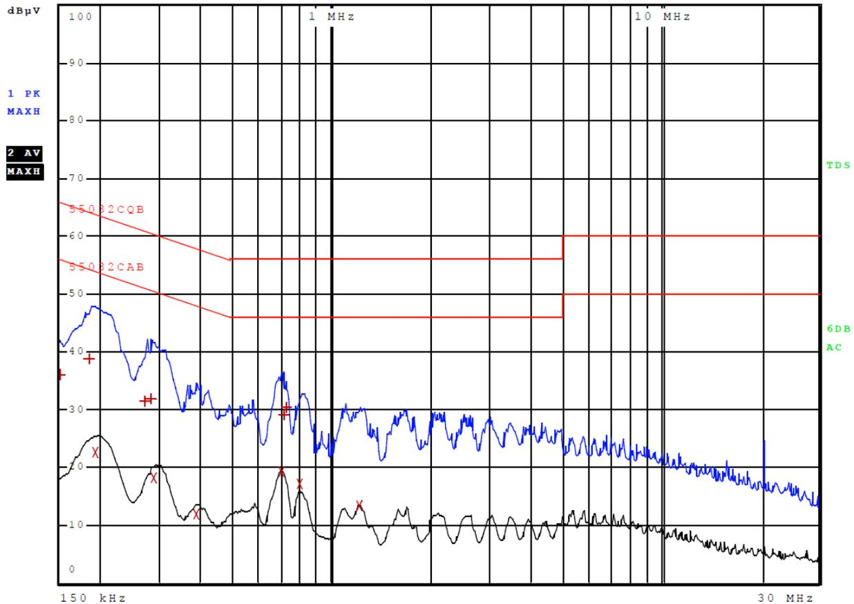
Figure 3 AC Line Conducted emissions of EUT line 1 (Configuration #3, EUT – 362-00087-00)
