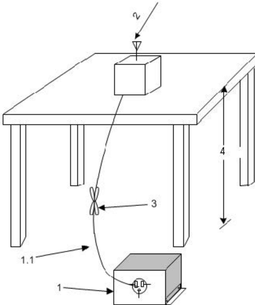
1—A LISN is optional for radiated measurements between 30 MHz and 1000 MHz but not allowed for measurements below 30 MHz and above 1000 MHz (see 6.3.1). If used, then connect EUT to one LISN. Unused LISN measuring port connectors shall be terminated in 50 Ω loads. The LISN may be placed on top of, or immediately beneath, the reference ground plane (see 6.2.2 and 6.2.3.2).
