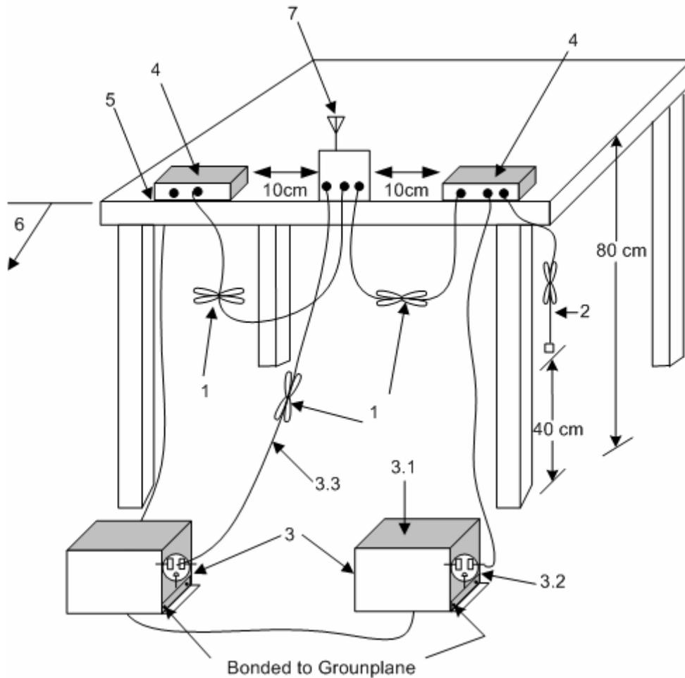
1. Interconnecting cables that hang closer than 40 cm to the ground plane shall be folded back and forth in the center forming a bundle 30 cm to 40 cm long see (see 6.2.3.1).
