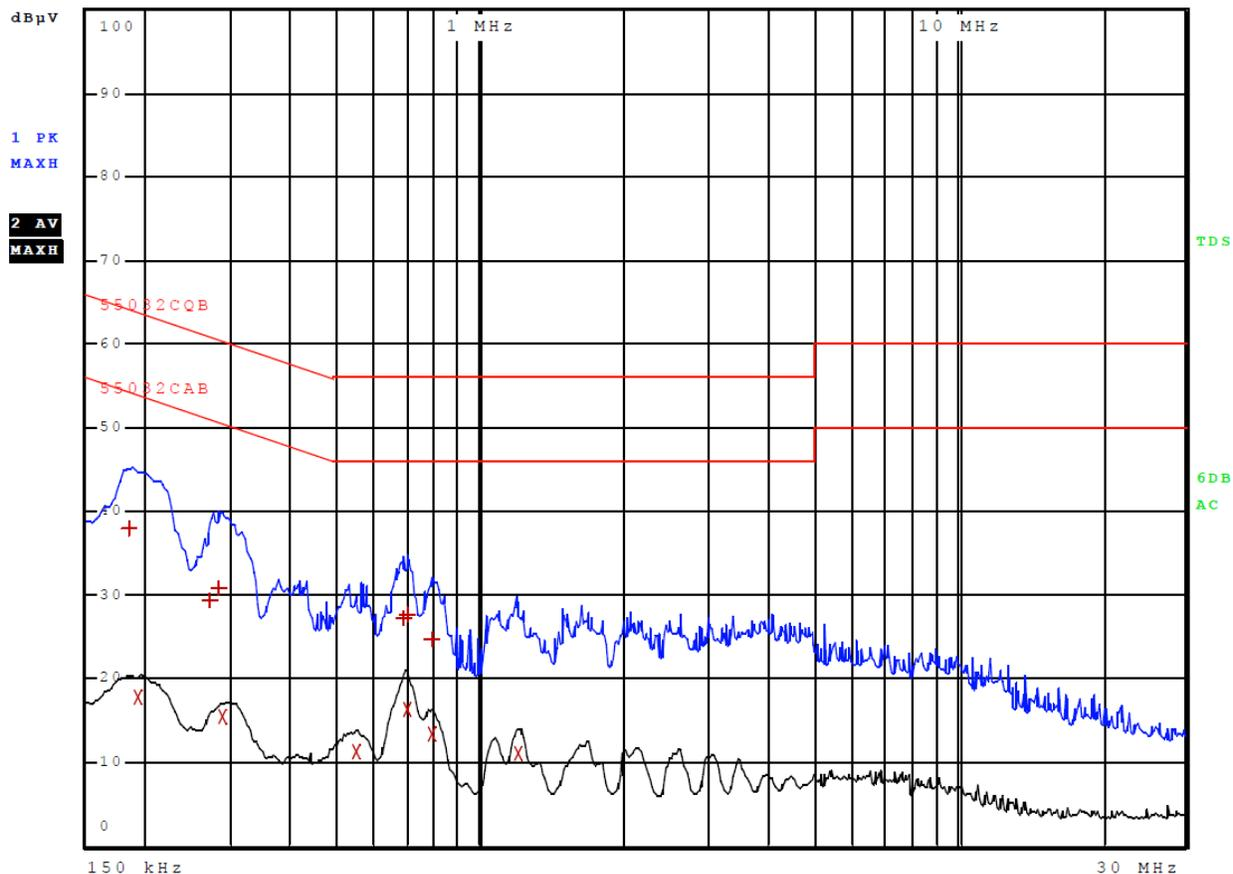
Figure 4 AC Line Conducted emissions of EUT line 2 (Configuration #3, EUT – 362-00087-00)
