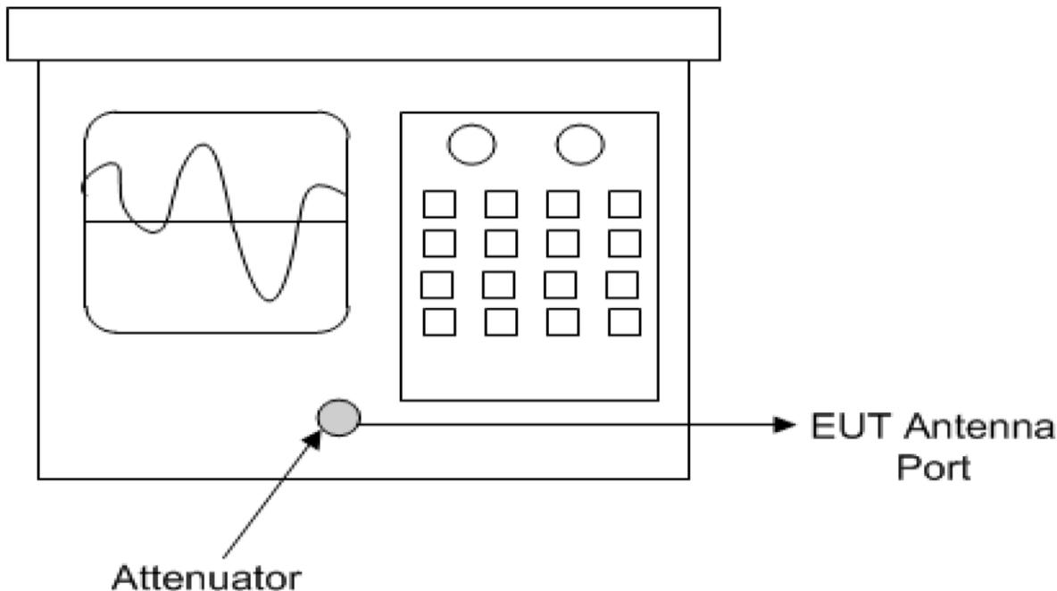
**Diagram 4 Test arrangement for Antenna Port Conducted emissions**
