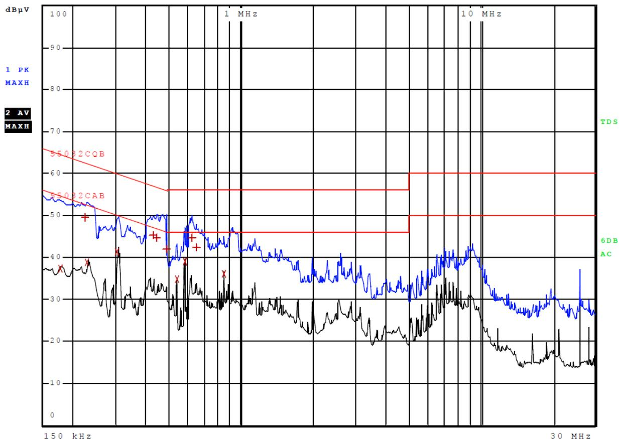
Figure 2 AC Line Conducted emissions of EUT line 2 (Configuration #2, EUT – Computer)
