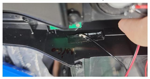
Tip: First fasten the terminal block and then tear the back tape antenna, the antenna must stick straight according to the drawing.thank you!
