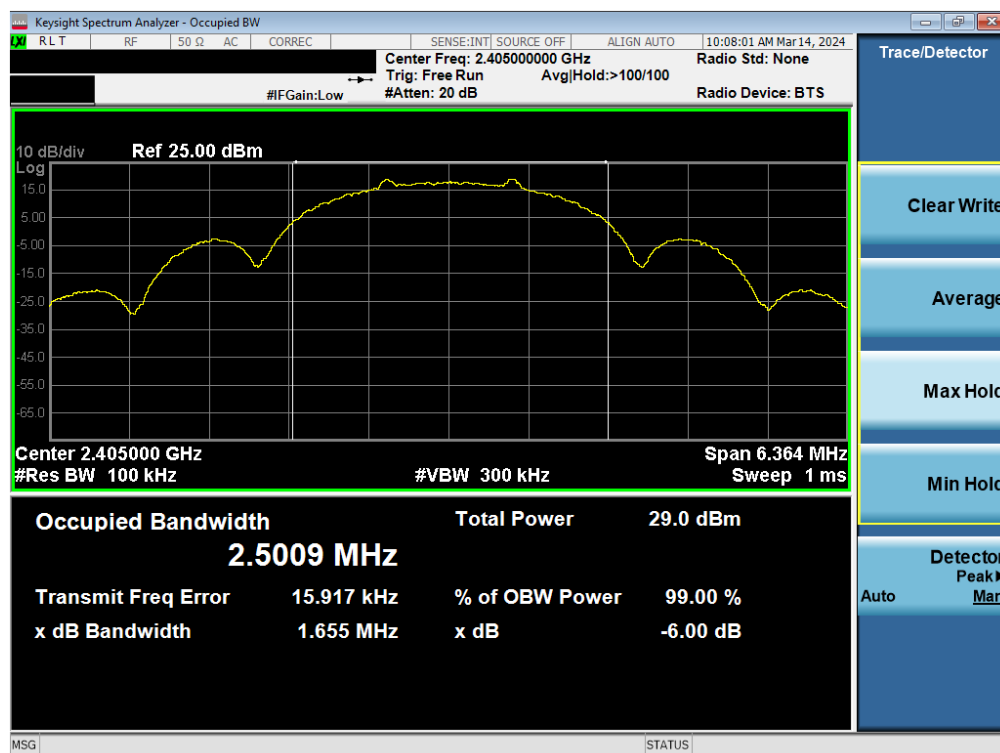
Plot 7-1. 6dB BW & 99% OBW Antenna WF7b (802.15.4, Ch. 11)
