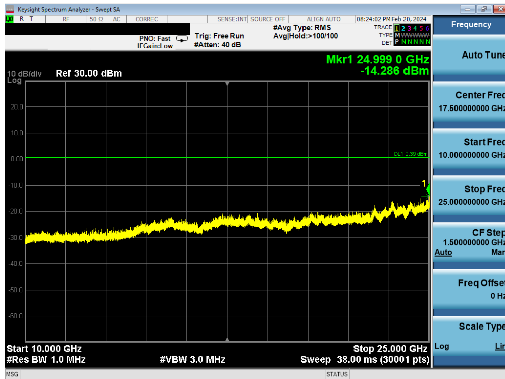
Plot 7-28. Conducted Spurious Antenna WF7b (802.15.4, ePA – Ch. 25)
