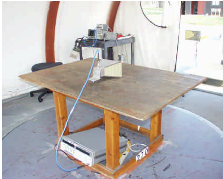
1 – 18 GHz Substitution Method Setup
