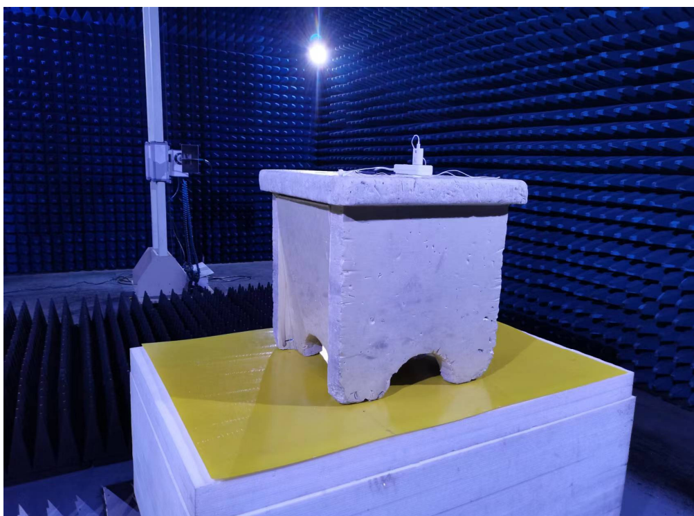
Photo of Radiated Emission Measurement (Above 1G)
