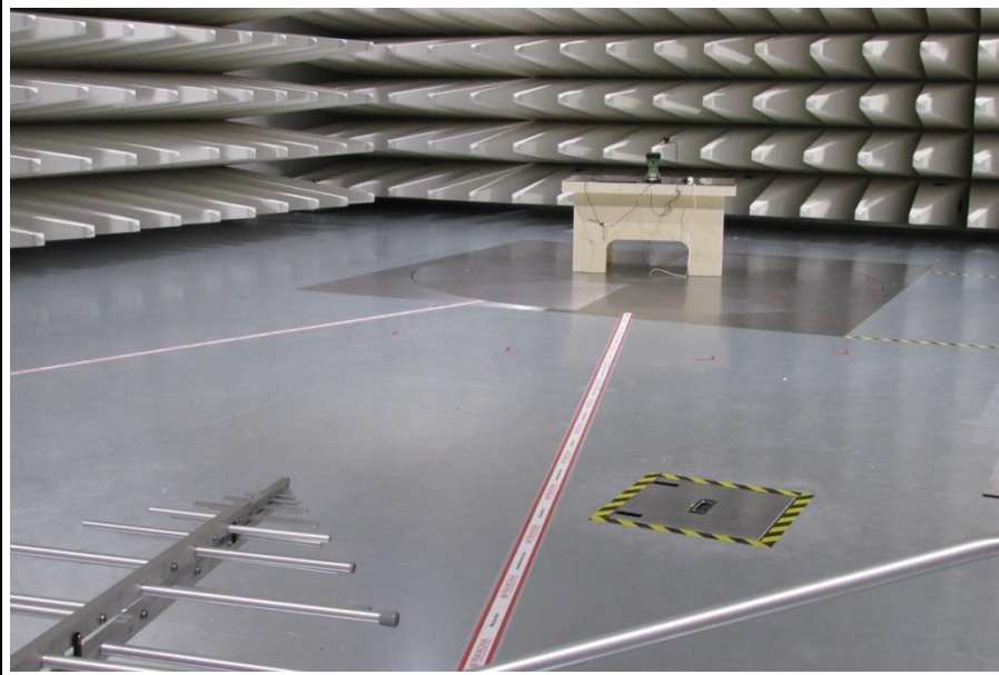
Test Setup : Radiated Emissions Docking Station
