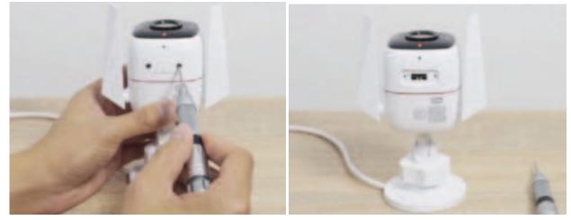
2. Identify the direction of the microSD card and carefully insert the card into the slot. Push in the card until you hear a clicking sound.
