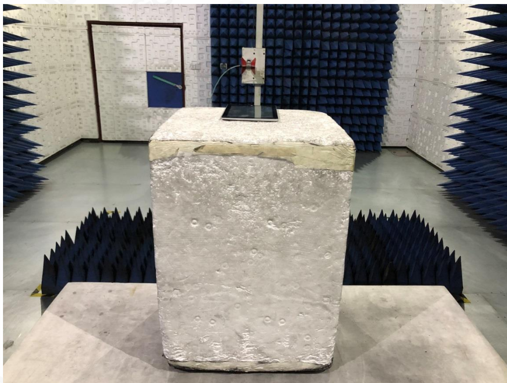
FCC RADIATED EMISSION TEST SETUP ABOVE 1GHZ
