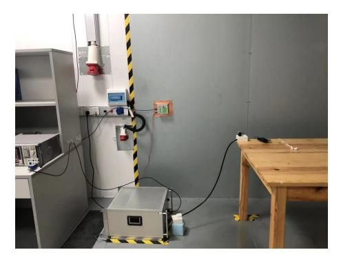
Set-up for Radiated Emission (RE), Below 1GHz
