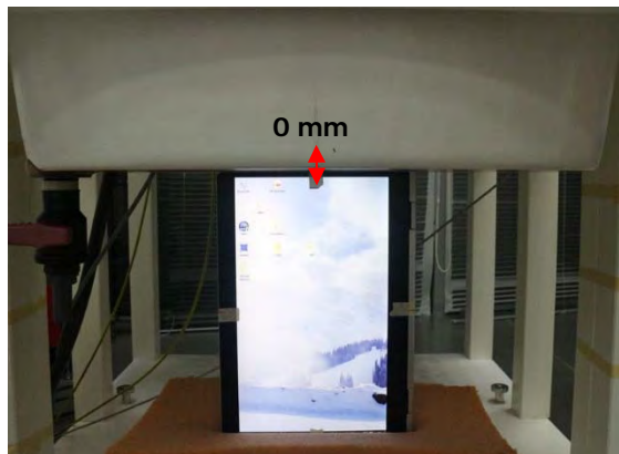
Fig.6 EUT Right side to flat phantom
