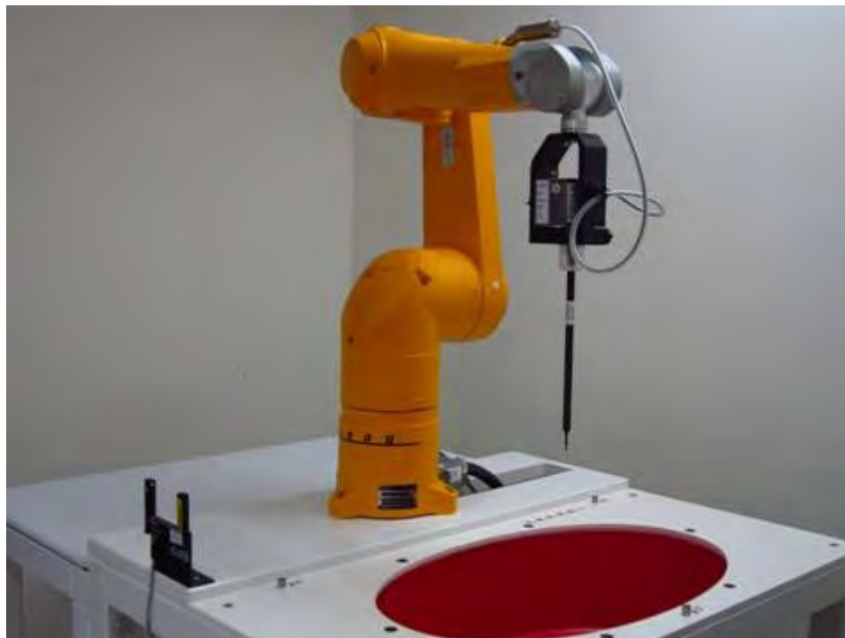
Fig.1 Photograph of the SAR measurement system
