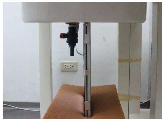
Fig.6 EUT Right side to flat phantom
