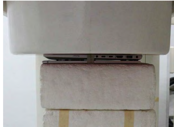
Fig.3 EUT Back side to flat phantom
