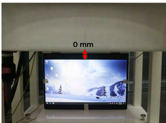
Fig.5 EUT Bottom side to flat phantom
