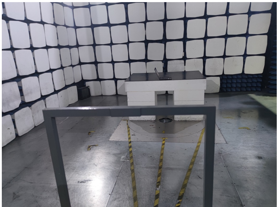
Radiation Emission Test Setup (Below 30MHz)
