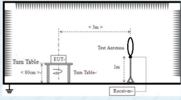
For radiated emissions from 30MHz to1GHz
