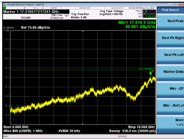
4-18 GHz, Vertical Antenna Flat EUT, Channel 19
