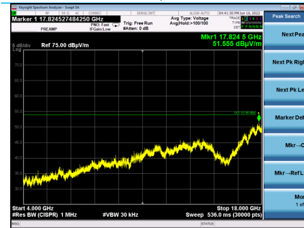
4-18 GHz, Horizontal Antenna Flat EUT, Channel 19
