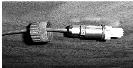
Figure 37. End Nut Seated on RJ45 Connector
