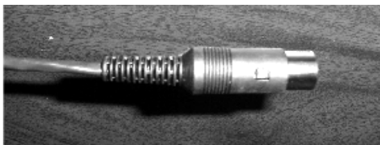
Figure 33. Jacket Placed Over 8-Pin DIN Connector
