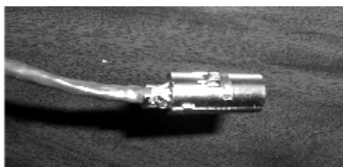
Figure 32. Metal Shell Placed Over 8-Pin DIN Connector
