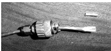
Figure 34. Cat 5 Cable with Insulation Removed
