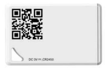
The TAG ID is necessary to provision the device. This information is encoded in the QR code.
