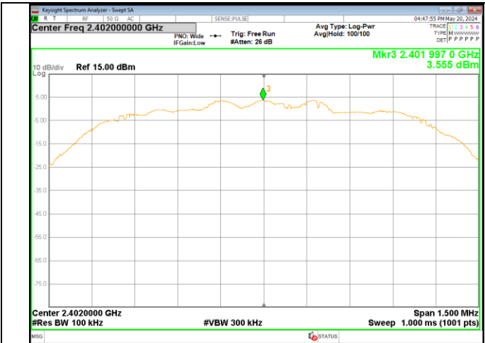
In-Band Reference Level 8DPSK_3-DH5_Channel 0
