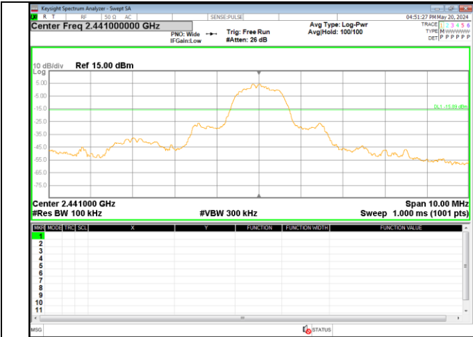
Out Of Band Emission 8DPSK_3-DH5_Channel 39
