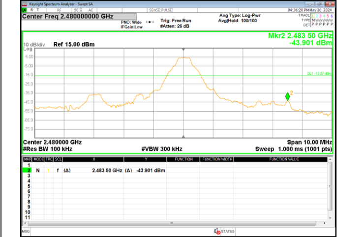
Out Of Band Emission GFSK_DH5_Channel 78
