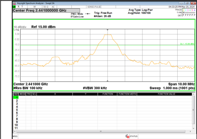
Out Of Band Emission GFSK_DH5_Channel 39
