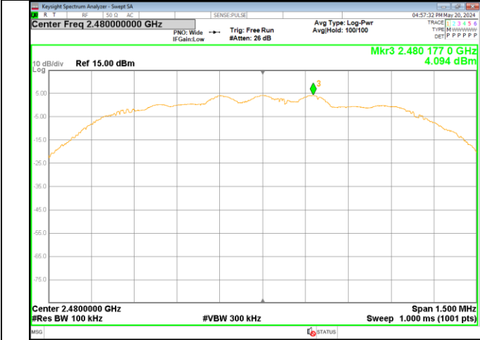
In-Band Reference Level 8DPSK_3-DH5_Channel 78
