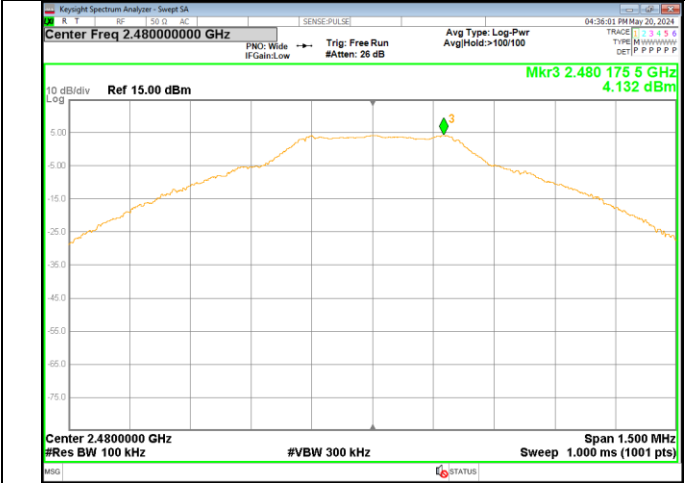
In-Band Reference Level GFSK_DH5_Channel 78
