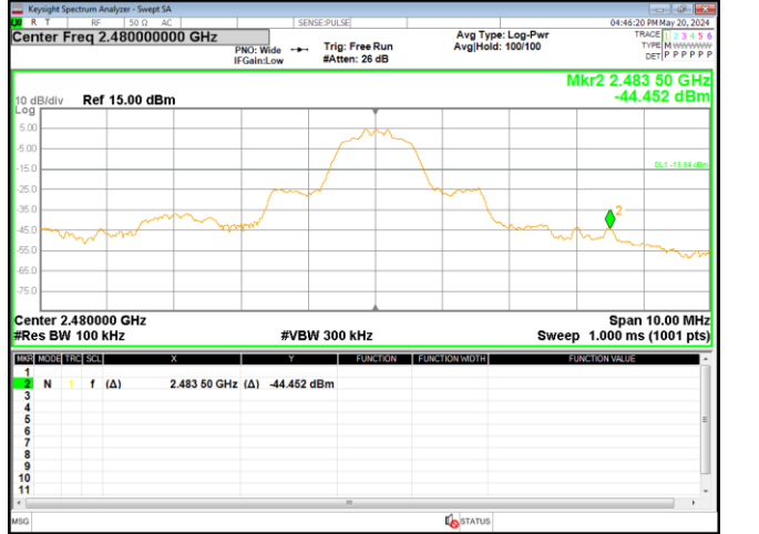
Out Of Band Emission \pi/4 DQPSK_2-DH5_Channel 78
