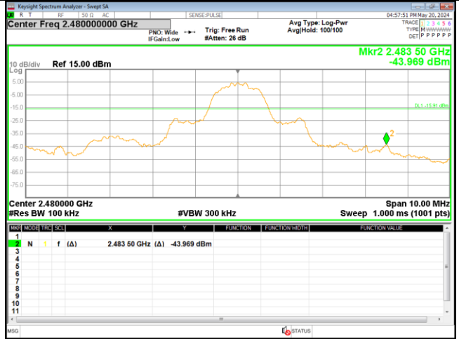
Out Of Band Emission 8DPSK_3-DH5_Channel 78
